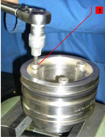
**1** Loosen allen screws and remove.
